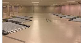
When using Autostacker parking systems, you'll find that you are able to store vehicles in a much tighter space than typically required for individual parking units. A normal parking stall requires around 300 – 350 square feet for the stall, plus a moderate amount of clearance for drive aisles. Autostacker's floor space requirement is just 200 square feet, and again, that delivers you two spaces, not just the one.
